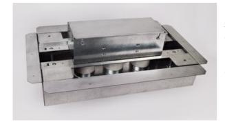
3-Gang Fire Classified Steel Floor Box. Adjustment range over deck of 2" (51mm) minimum to 5" (127mm) maximum. Three 1 1/4" (32mm) conduit feed openings. Inside Gang Capacity - 67.5 cubic inches. Outside Gang Capacity - 54 cubic inches each gang. This floor box preserves the 2-hour fire rating of floors in which it has been installed.
