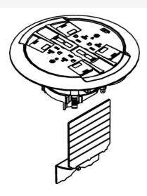
For 881PVC Floor Box. Kit complete with two (2) 20A duplex receptacles, (receptacles can be wired as standard or Isolated Ground), flange and slide holder, 881ADP Adapter, and 881DIV Divider. Provided with Wiremold CM Series Open System unloaded adapters, Ortronics Series II and TracJack adapters. Modular jacks sold separately. CAUTION: Not for use on concrete pours less than 4 1/2" (114mm) deep. Not for use when concrete is the finished floor. Use only for tile, carpet, or wood covered floors.
