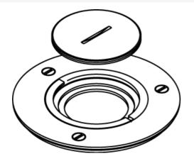
Brass communications or power cover plate with 2 1/4" (57mm) threaded opening for tile. NOTE: For carpet or tile installations. All cover plates are furnished with gasket and three screws. The 895P Polycarbonate Series Cover Plates must be field modified for dual service.
