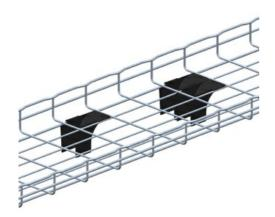
Use Bottom Drop Out for smaller groups of cables that are entering and exiting Cablofil Cable Management. Its smooth, high-density plastic construction eliminates deformation and damage to cable bundles. Bottom Drop Out snaps into any bottom opening without the need for attachment hardware.
