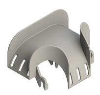
Use Over-the-Top Waterfall for cables that exit or enter the side of the tray. It eliminates the need to cut any side wires that reduce tray integrity. Over-the-Top Waterfall features steel, powder coated construction and hold-down slots to zip tie cables in place.
