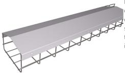
Stainless steel snap on peak cover for wire mesh tray 316L, 4"" width. Food and beverage processing plants are often harsh, challenging environments that demand extra consideration when it comes to equipment. With frequent washdowns and exposure to chemicals, stainless steel options are ideal due to their durability and resistance to corrosion. Stainless steel cable tray and accessories are easy to install, clean and meet National Sanitation Foundation standards.
