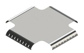
Junction bridges keep cables separated at tees and crosses in Cablofil cable management for optimum network signal integrity. The unique design creates smooth cable transitions to keep cables from kinking and bunching. Bridges mount in place using a BC1 Bridge Clip bolted to CE35 or EZT90/RADT90 junction hardware. Each bridge is predrilled with BH75 Bridge horn mounting holes and slots to secure cables with nylon zip ties.
