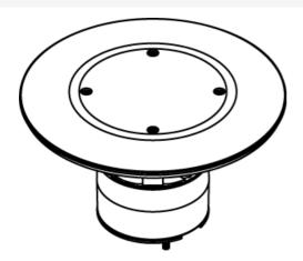
Complete plug assembly for abandoning an open 3" (76mm) diameter hole. Assembly includes intumescent fire-stop material to maintain the fire-classification of the floor, integral retainer ring to prevent the unit from pulling up through the floor, and a black diecast aluminum cover.
