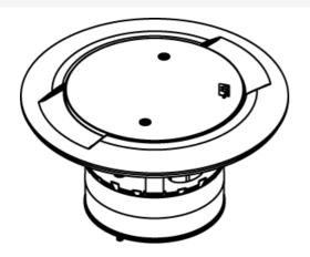
Complete plug assembly for abandoning an open 4" (102mm) diameter hole. Assembly includes intumescent fire-stop material to maintain the fire-classification of the floor, integral retainer ring to prevent the unit from pulling up through the floor, and a black diecast aluminum cover.
