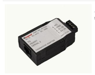
This adapter facilitates communication between Unity Integration Module and RCS-TR60 thermostat.
