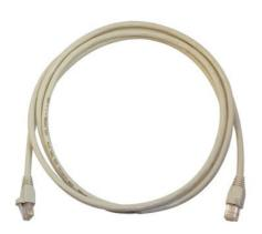
This component-rated 500 MHz Cat 6a patch cable is designed to fully support 10 Gigabit Ethernet speeds up to 100 meters. The snagless boot protects the tab from catching on other cables in high-density patch panel applications, ensuring a smooth and efficient setup. ETL verified to support the Cat 6a performance specification, this patch cable exceeds 750 insertion cycles as specified in FCC part 68 Subpart.
