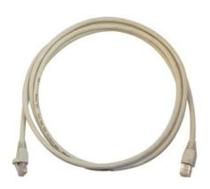
This component-rated 500 MHz Cat 6a patch cable is perfect for high-density patch panel applications, fully supporting 10 Gigabit Ethernet speeds up to 100 meters. The snagless boot design protects the tab from catching on other cables, ensuring a hasslefree setup. ETL verified to support the Cat 6a performance specification, this patch cable exceeds 750 insertion cycles as specified in FCC part 68 Subpart.
