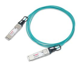
25m Avago/Broadcom AFBR-7QER25Z Compatible 40GBase-AOC QSFP+ to QSFP+ (MMF, 850nm, LSZH) Active Optical Cable
