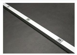
Available in 3' (914mm) length with 12" spacing. USB is 2.4 Amps (shared between two ports) 5VDC. .040" (1.0mm) aluminum housing. Packed two per carton. Each unit supplied with one (1) Coupling and two (2) Blank End Fittings.
