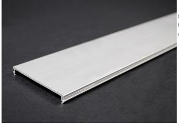
6063-T5 extruded aluminum, satin anodized finish. Nominal wall thickness .060'' (1.5mm). Packed eight 5'(1.5m) lengths per carton. Made in U.S.A.
