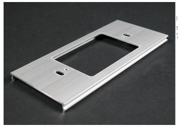
Installs communication connectivity devices utilizing the industry standard single-gang faceplates. Hole cut is 2'' x 2 7/8'' (51mm x 73mm). Faceplates must be ordered separately.
