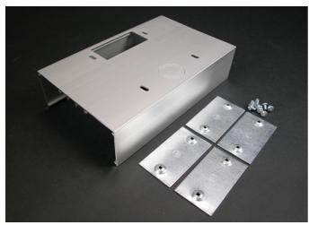
Feeds raceway from a wall-mounted outlet box. Rectangular hole cut or concentric 1/2" and 3/4" trade size Kos. Couplings included.
