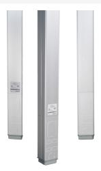
Two-compartment pole. Nominal material thickness .050" [1.8mm]. Length: 10' 5" [3.2m]. Furnished unwired without outlets. Two 8" [203mm] removable covers with KOs for modular jacks and modular furniture communication outlets. Mounting hardware, entrance end plate and ceiling trim plates furnished. NOTE: Custom options - features such as colors or other lengths [20' [6.1m] maximum] available on custom orders.
