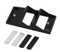
For use with multi-channel raceway device brackets and WallSource device mounting brackets. Angled exit provides additional mounting depth required for A/V connections as well as ensuring the required bend radius for UTP and fiber optic cabling. Holds two Ortronics Series II modules. Fits 5507 Series Faceplate opening. Fits 5507 Series Faceplate opening.
