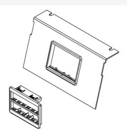
For AC8850 Box. Includes two (2) Ortronics Series II and two (2) TracJack adapters. NOTE: AC8850 is a single-service box. Power plates cannot be used in conjunction with communication plates.
