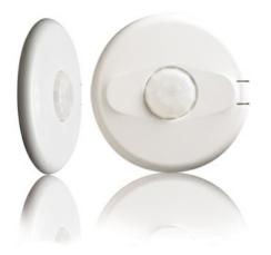
Wattstopper's CI-355 passive infrared (PIR) occupancy sensor automatically turns lighting on and off based on occupancy. The sensor mounts on the ceiling with a flat, low-profile appearance and provides 360 degrees of coverage.
