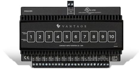
The DIN Contact Input Station is part of Wattstopper's Architectural Dimming system and provides a single integration point for a large variety of sensor inputs and external switches. Each station features ten contact input channels for monitoring the open and close states from a variety of external devices. These devices include magnetic door contact switches, momentary switches, motion detectors, daylight sensors, and more.
