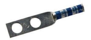
Size 6 cable, .625 inches on center between holes, 1/4 inch screw size, blue. Manufactured from electroplated tinned copper. Long barrels maximize number of crimps and are color coded. Inspection port assures full conductor insertion. 10pk.
