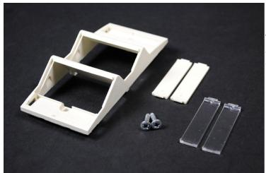
For use with multi-channel raceway device brackets and WallSource device mounting brackets. Angled exit provides additional mounting depth required for audio/visual connections as well as ensuring the required bend radius for UTP and fiber optic cabling. Holds two CM2 Series modules or two CM2 Series modules or two 2A inserts. Fits 5507 Series Faceplate opening.
