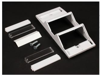
For use with multi-channel raceway device brackets and WallSource device mounting brackets. Angled exit provides additional mounting depth required for audio/visual connections as well as ensuring the required bend radius for UTP and fiber optic cabling. Holds two CM2 Series modules or two CM2 Series modules or two 2A inserts. Fits 5507 Series Faceplate opening.
