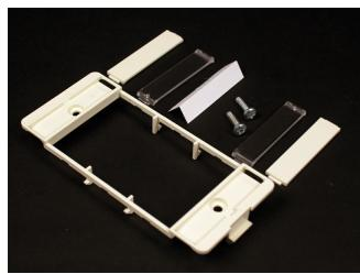
End plates with two outlet ID labels with clear covers and two matching screw covers. Required when mounting modules into 4050, 5450, 5550, and WSA07-4A device mounting brackets, and the V2444D-2Aand 2344SD-2A 2-gang divided raceway box.
