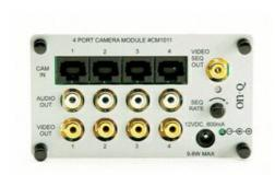
This Cat 5-based camera module supports up to four On-Q cameras and allows on-board sequencing of up to four images.
