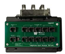
The 10x8 combo distributes up to 4 incoming telephone lines (RJ45) to 10 locations, and 1 GHz video to eight locations. The innovative mounting bracket includes a detachable platform for the coax splitter, allowing easy access to all termination ports
