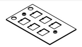
The CRFB4 has four compartments that accept different device plates. This Communication Plate is for Plate location 4, with six (6) RJ knockouts. Modular jacks sold separately. NOTE: Standard size for device plates for Plate Location 2 is 5 7/32" [132mm] x 2 3/4" [62mm].
