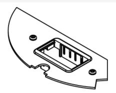
The CRFB4 has four compartments that accept different device plates. This Communication Device Plate is for Plate location 2, accepts two (2) ports of communication devices. Includes one (1) Wiremold CM Series Open System adapter and inserts. NOTE: Standard size for device plates for Plate Location 2 is 5 7/32" [132mm] x 2 3/4" [62mm].
