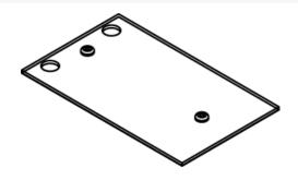
The CRFB4 has four compartments that accept different device plates. This Blank Device Plate is for Plate location 4, used to close off unused gang. NOTE: Standard size for device plates for Plate Location 4 is 5 7/32'' (132mm) x 2 3/4'' (62mm).
