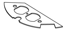
The CRFB4 has four compartments that accept different device plates. This Duplex Device Plate is for Plate location 1, accepts standard 15A and 20A duplex receptacles. NOTE: Standard size for device plates for Plate Location 1 is 6 11/32" [161mm] x 2 3/4" [62mm].
