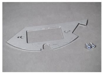
The CRFB4 has four compartments that accept different device plates. This GFCI/Decorator Device Plate is for Plate location 1, accepts standard GFCI or Decorator style receptacles. NOTE: Standard size for device plates for Plate Location 1 is 6 11/32'' [161mm] x 2 3/4'' (62mm].
