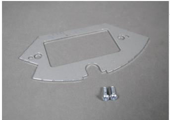
The CRFB4 has four compartments that accept different device plates. This GFCI/Decorator Device Plate is for Plate location 3, accepts standard GFCI or Decorator style receptacles. NOTE: Standard size for device plates for Plate location 3 is 6 11/32" (161mm) x 2 3/4" (62mm).
