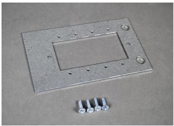
The CRFB4 has four compartments that accept different device plates. This Device Plate is for Plate location 4, holds four (4) Legrand AVIP or Extron Electronics MAAP device plates. NOTE: Standard size for device plates for Plate Location 4 is 5 7/32'' (132mm) x 2 3/4'' (62mm).
