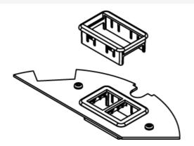
The CRFB4 has four compartments that accept different device plates. This Communication Device Plate is for Plate location 1, accepts two (2) ports of communication devices. Includes one (1) Ortronics Series II and one (1) Tracjack adapter. NOTE: Standard size for device plates for Plate Location 1 is 6 11/32" [161mm] x 2 3/4" (62mm).
