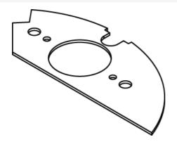
The CRFB4 has four compartments that accept different device plates. This Device Plate is for Plate location 2, accepts most 20A and 30A turnlok receptacles. NOTE: When using a 30A device, egress opening must be located directly over receptacle. Standard size for device plates for Plate Location 2 is  $5\,7/32$ " (132mm) x  $2\,3/4$ " (62mm).
