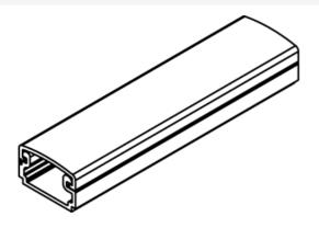
Tunnel allows the two outer compartments to be utilized for one service while the center two compartments are utilized for other services.
