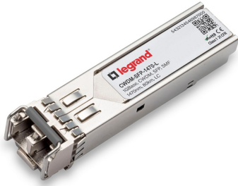
Cisco CWDM-SFP-1470 Compatible 1000Base-CWDM SFP Transceiver (SMF, 1470nm, 80km, LC Duplex, DDM, I-Temp)
