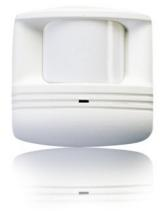
The CX-105 Passive Infrared (PIR) Ceiling/Wall Sensors detect occupancy to control lighting in a dense, wide-angle coverage pattern up to 2000 sq ft (185.8 sq m). This model does not include an isolated relay for integration with BAS or HVAC.
