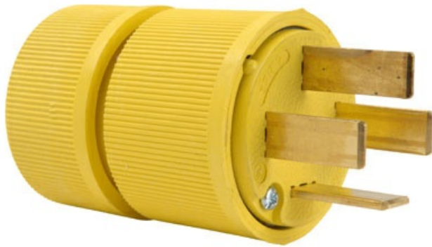
Gator Grip Plug, 4 pole 4-Wire, 60A 120/208V, Yellow
