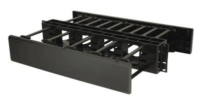
Legrand® standard horizontal cable managers are available in 1RU and 2RU sizes. Fingers begin 3/4" from the face of rack to provide bend limitation for cables, protecting cables, equipment and network performance. Included hinged cover mounts with six heavy duty clips allow them to be opened one handed without becoming "unhinged". Manufactured from UL94V-0 rated plastic.
