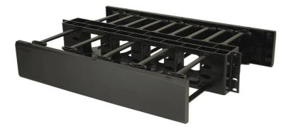
Legrand® standard horizontal cable managers are available in 1RU and 2RU sizes. Fingers begin 3/4" from the face of rack to provide bend limitation for cables, protecting cables, equipment and network performance. Included hinged cover mounts with six heavy duty clips allow them to be opened one handed without becoming "unhinged". Manufactured from UL94V-0 rated plastic.
