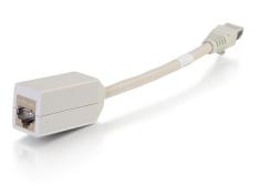
Quick release device protection adapters protect IT equipment and eliminate trip hazards by reducing pull-out force for applications that require a hard wired connection to the LAN. Backward compatible to Cat6 and Cat5e.
