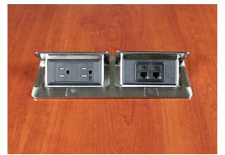
Unit includes one (1) 15A black tamper-resistant duplex receptacle. Second opening will accept adapter for one (1) Wiremold CM Series Open System 2A module, one (1) Ortronics Series II or one (1) TracJack adapter to accommodate a wide range of communication outlets. Adapters are included in hardware bag. Unit comes with a 6' (1.83m) cord. Comes with a brushed stainless steel finish.
