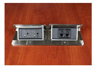
Unit includes one (1) 20A black tamper-resistant duplex receptacle. Second opening will accept adapter for one (1) Wiremold CM Series Open System 2A module, one (1) Ortronics Series II or one (1) TracJack adapter to accommodate a wide range of communication outlets. Adapters are included in hardware bag. Unit comes with a 6' (1.83m) cord. Comes with a brushed stainless steel finish.
