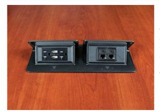
Unit includes one (1) 20A black tamper-resistant duplex receptacle with two (2) USB ports that provide 3.1A. Second opening will accept adapter for one (1) Wiremold CM Series Open System 2A module, one (1) Ortronics Series II or one (1) TracJack adapter to accommodate a wide range of communication outlets. Adapters are included in hardware bag. Unit comes with a 6' (1.83m) cord. Comes with a black powder coat finish.
