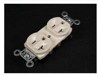
Specification grade rated 20A 125V NEMA 5-20R receptacle. Receptacle has nylon face and thermoplastic base. One-piece brass triple-wipe line contacts and double-wipe ground contacts. Locked in wrap-around steel yoke. Break off tab for two circuit wiring. 2.7" W x 4.5" H (69mm x 114mm). Verified under Fed. Spec. #WC596F.
