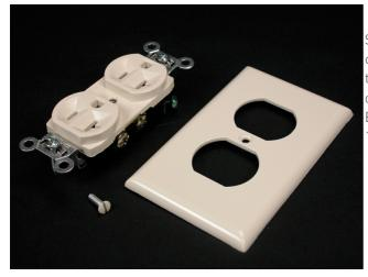
Specification grade rated 20A 125V NEMA 5-20R receptacle with color matched nylon faceplate. Receptacle has nylon face and thermoplastic base. One-piece brass triple-wipe line contacts and double-wipe ground contacts. Locked in wrap-around steel yoke. Break off tab for two circuit wiring. 2.7'' W x 4.5'' H (69mm x 114mm). Verified under Fed. Spec. #WC596F.
