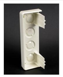
Closes off end runs of 5400 Series Raceway. Has four  $1/2^{\prime\prime}$  trade size KOs for end feed.
